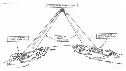
Fig. 17. Power relay satellite concept {Kraft-Ehricke, 1973} [44].
