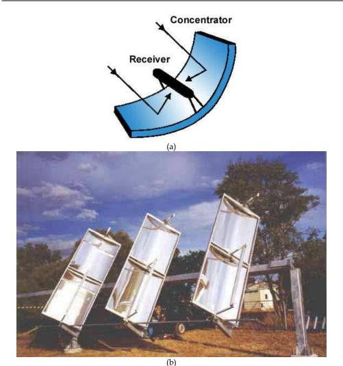
Fig. 22. (a) Schematic of a parabolic trough concentrator. Image adapted from Energy Efficiency Renewable Energy Network {Council of Australian Governments, 2006} [63]. (b) Trough concentrator system at the Australian National University, which is designed to incorporate photovoltaic power generation or water heating and steam production. (Image courtesy of the Centre for Sustainable Energy systems, Australian National University, {Wyld Group, 2009} [64].
