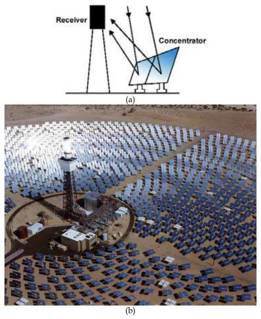
Fig. 21. (a) Schematic of a power tower. Image adapted from Energy Efficiency Renewable Energy Network {I. Tidwell, 2005} [61];
