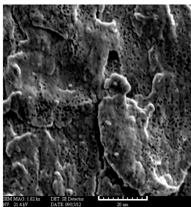
FIGURE 7. Surface of Ni on which Cu was deposited after heating in vacuum at 481° C.
