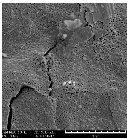
FIGURE 8. SEM image of a surface of Ni on Pd after the study containing voids and cracks.
