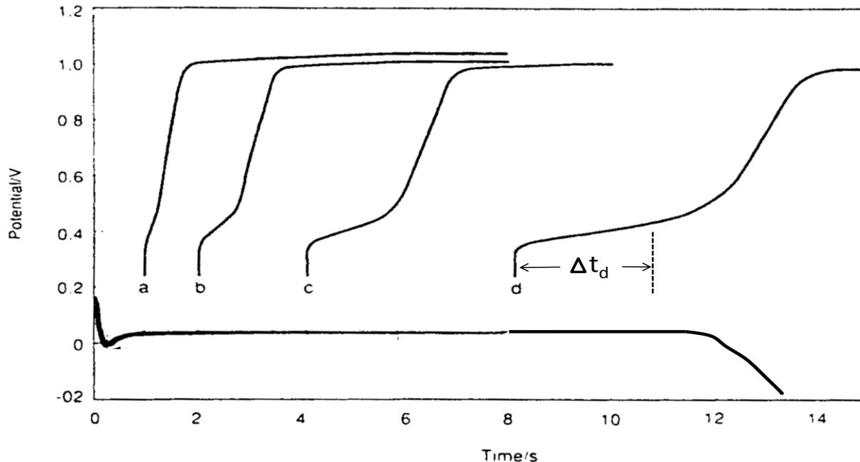
Deuterium up-take during co-deposition.  $j_c = -5 \text{ mAcm}^{-2}$  and  $j_a = 5 \text{ mAcm}^{-2}$ , with cell current reversal at 1, 2, 4, and 8 seconds.
