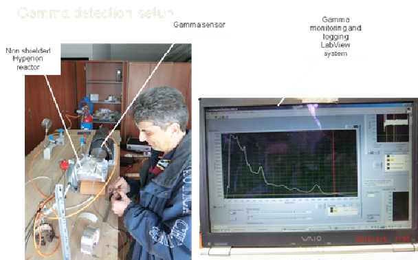
Fig. 4. Hyperion gamma detection setup
